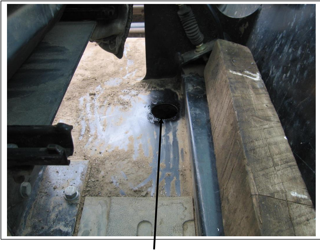
Drill a 2 1/2" hole in the floor for the A/C hoses, drain tubes and wiring. Install edging around the hole to protect the hoses.
