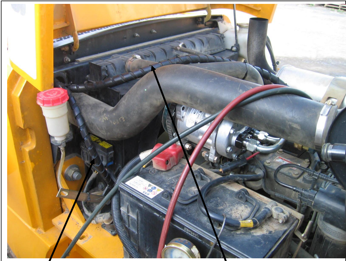
5/16" line running from the condenser to the drier.
