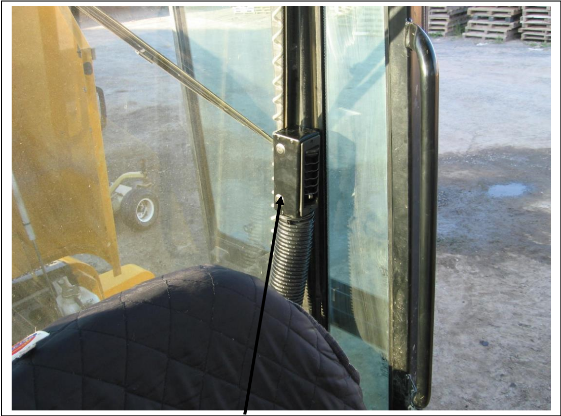
Remote mount louver box screwed to rear post of cab.
